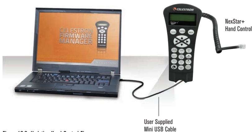
Figure 12.2 Updating Hand Control Firmware
